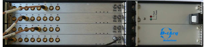
Fig. 4. Four ACQ216CPCI Digitizer Boards from D-TACQ enable parallel data acquisition for 32 receiver channels.
